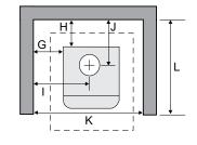
**RESIDENTIAL CLOSE CLEARANCE (TO BE INSTALLED WITH REQUIRED PIPE COMPONENTS)** When the stove is installed as a close clearance residential unit, a listed double wall connector is required from the stove collar to the ceiling level.
