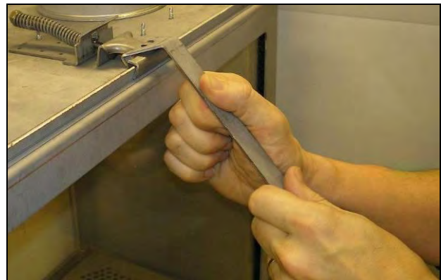
Step 4: Draw Latch forward with other hand.
