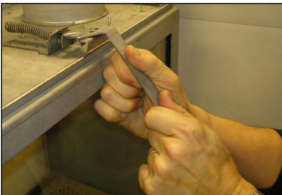
Step 5: Release Latch from Door.
