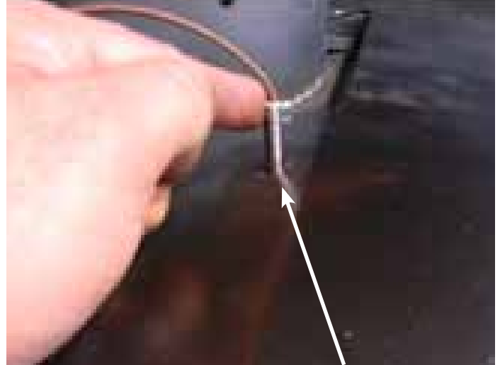
Install temperature probe
