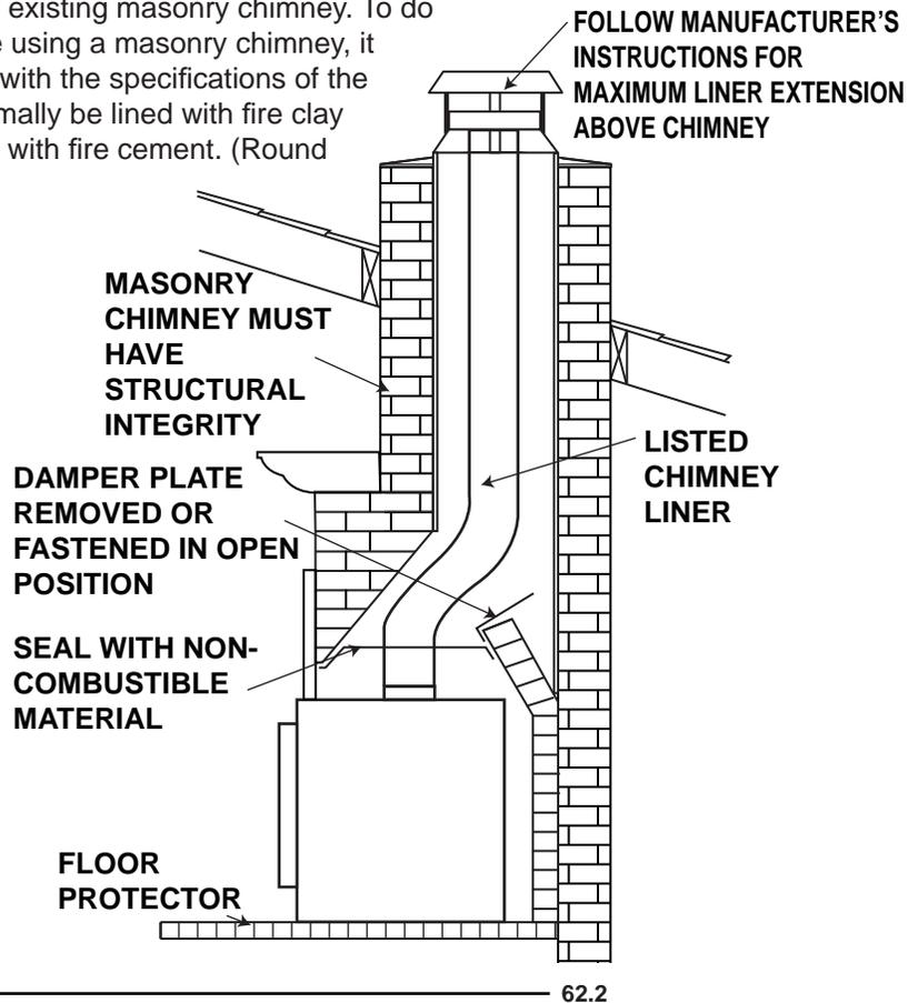
**A.** Remove the fireplace damper or fasten it permanently open.
