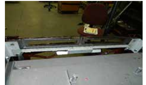
Lift light assembly bracket off bolts to install bulb Remove two screws in locations shown
