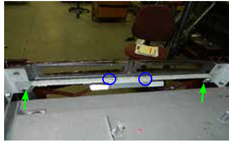
Lift light assembly bracket off bolts to install bulb Remove two screws in locations shown
