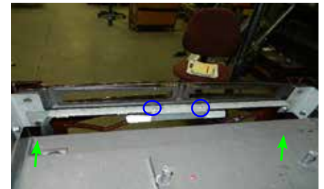
Lift light assy bracket off bolts to install bulb
