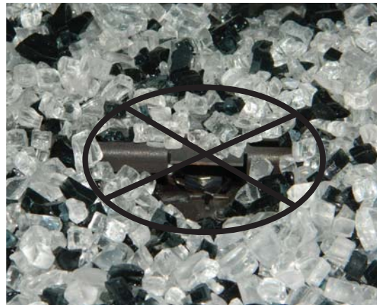
DO NOT block pilot area with glass crystals
