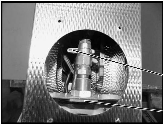
Figure 13: Gas on-off valve.
