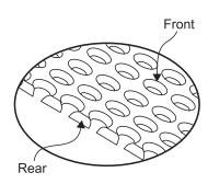
Note: The grill has a front and rear, the holes on the front side have rounded edges and the rear holes have flat edges.
