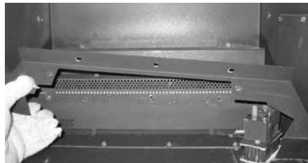
Burner Tray Removed
