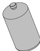
**WARNING!** The dust cap should be in place when the propane cylinder is not in use to prevent dirt and debris from entering.
