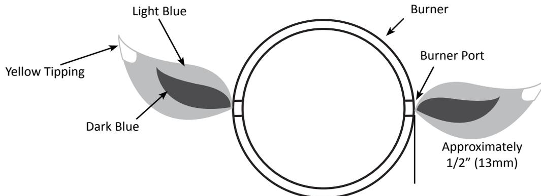
**Combustion Air Adjustment:** (This must be done by a qualified gas installer.) The air shutter is factory set and should not need adjusting under normal conditions. Under extreme field conditions, adjustments might be required. When the air shutter is adjusted correctly the flames will be dark blue, tipped with light blue and occasionally yellow.
