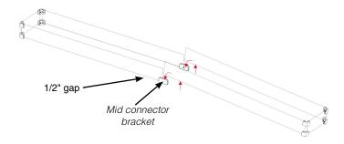
Use the supplied jig to support the 2 glass sections when installing the Mid connector bracket-this will keep the 2 glass sections level
