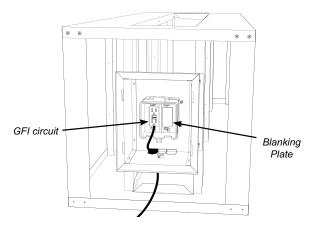
5. Plug in the supplied AC adaptor and run the wire through the bottom of the outer box, be sure to use a grommet to protect the wire.
