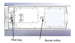
Remove burner orifice with a 1/2" wrench. Use another wrench to hold on to the elbow behind the orifice. Discard orifice. Install new NG orifice supplied with kit.
