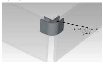
**4a.** After the 2 top brackets are installed--gently flip over both sides over and place on a soft surface, to install the 2 bottom brackets on each side
