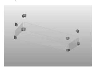
**4b.** Use supplied spacer tool to determine where the bottom bracket should be placed and secured.
