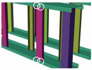
Diagram 8- Outside vertical supports (B1) with screws locations
