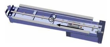
7. Remove 8 screws on valve access cover.
