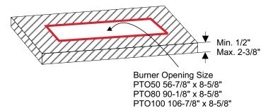
Important Note: Two (2) ventilation grills, (PTO50), Four (4) ventilation grills (PTO80 & PTO100) are highly recommended for all enclosures. This is to alleviate moisture and allow for air to circulate.
