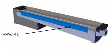
Side nailing strips are adjustable in 1/4" or 1/8" increments. Each hole on the inside line is 1/8", each hole on the outside line is 1/4" Determine the thickness of the finishing material before adjusting the nailing strips.
