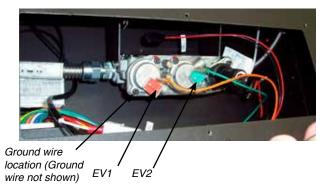
11. Remove 10 screws securing valve assembly.
