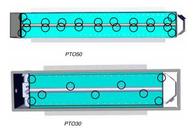
3. Lift burner tray off-burner tube can remain in place.
