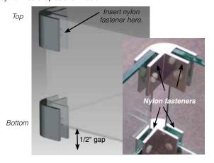
7. Set the mid connector brackets in between the 2 assembled glass wind-shields horizontally as shown below. Lift each end independently and slide into position in the bracket. When the tops of both sections are even, tighten the 2 Phillips head screws located on the mid connector. Maintain the 1/2" gap between the glass and the table top throughout the glass surround.
