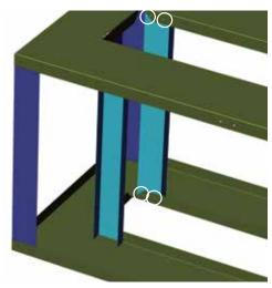
Diagram 6 - Inside vertical support (B2) screw locations
