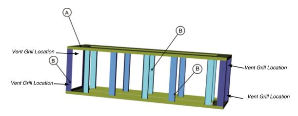
**Note:** For the 100" burner - Four (4) ventilation grills are required for all enclosures when joining two PTO50s together. This is to alleviate moisture and allow for air to circulate. Minimum recommended size 20"sq (508mm²) ea. The ventilation grills must be located at the ends of the burner in locations shown above.
