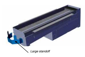
2. Remove 22 screws (PTO50) or 9 screws (PTO30) in locations shown below to remove burner tray (remove from both units).
