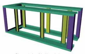
Diagram 5 - Install Inside vertical supports
