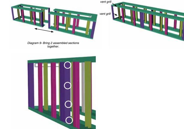
Diagram 10- Secure sections together with 4 screws through both inner corner Part Bs
