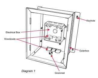
Install electrical box into the outer box with 4 screws.
