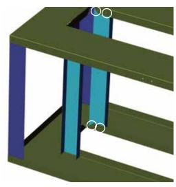
Diagram 5 - Inside vertical support screw locations
