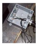
6. Attach low voltage wires to the switch - ensure to attach on the right side of the switch. This will make it easier to remove the 2nd battery terminal when replacing batteries. Fasten switch to right side of electrical box as shown below.
