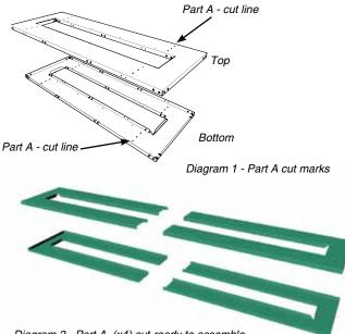
Diagram 2 - Part A (x4) cut-ready to assemble
