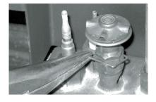
Pull off the pilot cap to expose the pilot orifice. Using a 5/32" allen key, remove pilot orifice and replace with LP pilot orifice.
