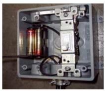
7. Install 4-AA batteries into each battery terminal. Ensure correct polarity. Slide the first battery terminal all the way to the right - until it is next to the switch. The 2nd battery terminal can be attached to the battery cover with the supplied velcro.
