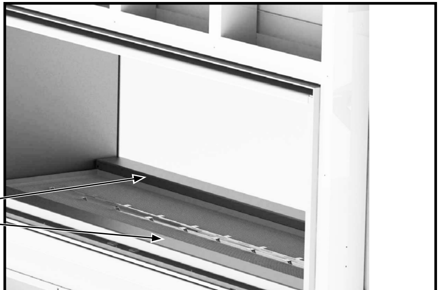
Figure 89: Installing porcelain strips.
